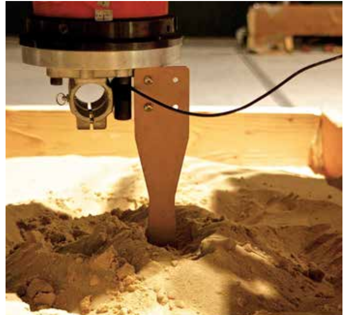
Fig. 3.7.4. Robot drives to dig around the placed object
