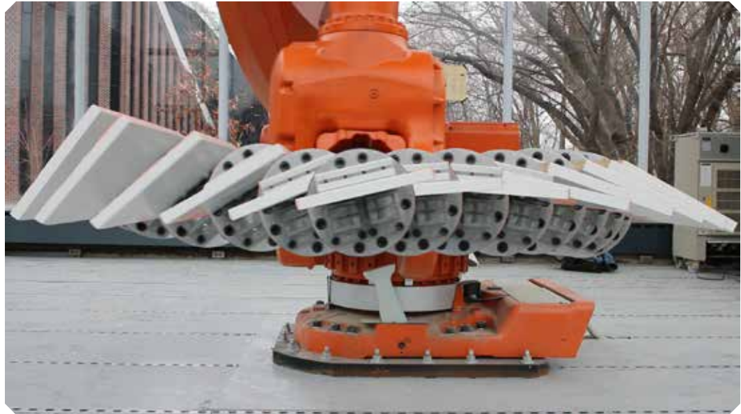
Fig. 3.16. The robot executes fluid, exaggerated movements generated by the physics simulation. In this particular simulation, it is clear that the rocking chair would have tossed a user off the chair to the left.
