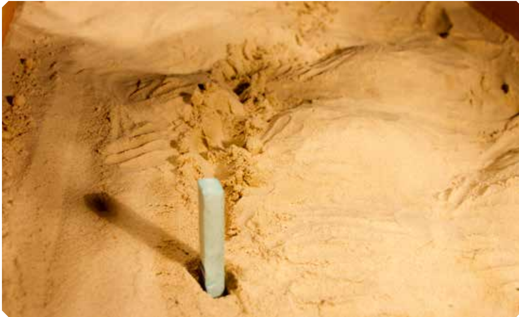
Fig. 3.11. The foam block is a tangible indicator for the computer to set the starting point of the road path simulation (photo by Charles Avis).
