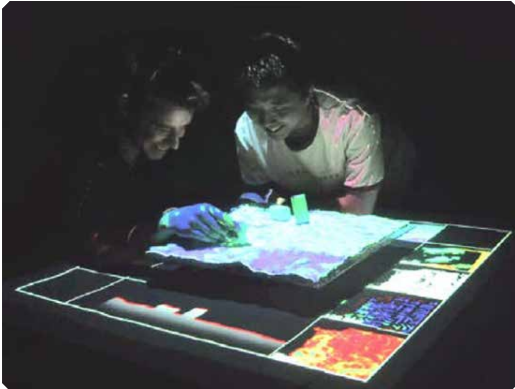
Fig. 3.1. SandScape from the Tangible Media Group at MIT. Projectors display GIS data on a scanned clay landscape (photo from Ishii et al , 2004)
