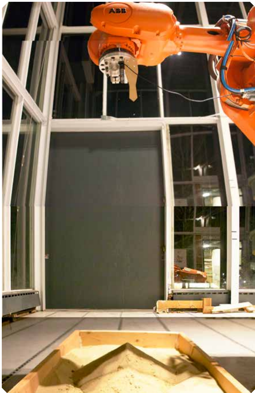
Fig. 3.3. The setup for SandCastle. The robot moves to this scan position, determines where it needs to go, then manipulates the sand with the wooden end-effector (photo by Charles Avis).
