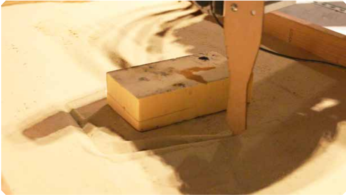
Fig. 3.5. A placed object, or even sculpted sand, will register as a human intervention, and the robot can act accordingly. Above is an example of the ‘moat’ algorithm that traces the outline of the sensed object (photo by Charles Avis).
