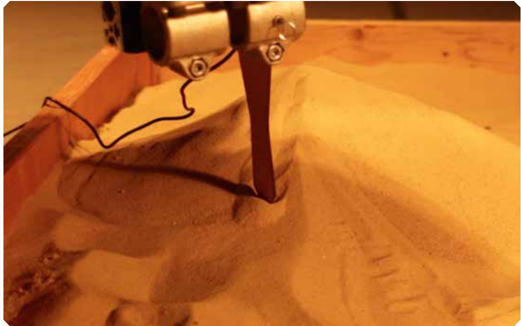
Fig. 3.10. The robot expressively tracing the calculated drainage line from the top of the mound (photo by Charles Avis)
