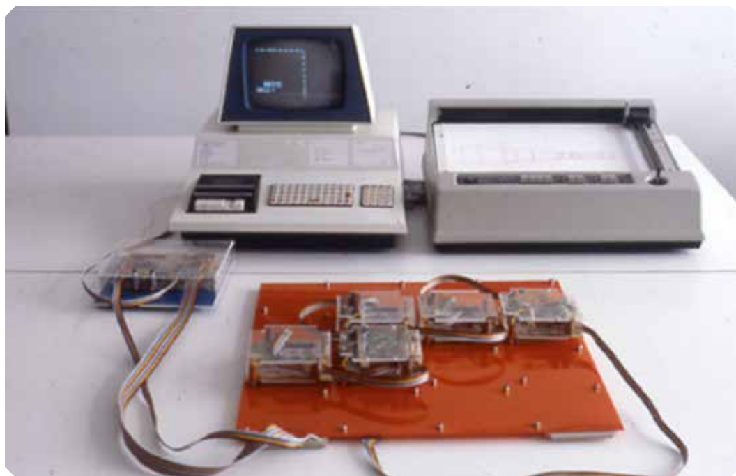
Fig. 2.7. John Frazer's prototype for Generator. The computer can read the positions of each block on the grid by polling the electrical connections between the grid, the blocks, and each block's neighbors (image from Cedric Price Archive, CCA).
