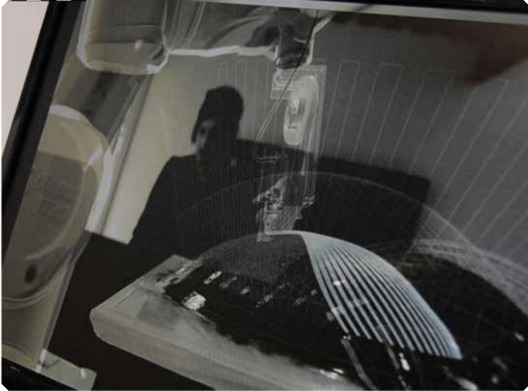
Fig. 1.7. Augmented Fabrication by Kruysmans and Proto is an animation-based simulation of robotic movements and tool paths. The synchronisation of robots, cameras, and digital simulations opens up possibilities for architectural applications beyond the mere making of objects.
