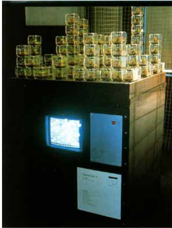
Fig. 2.9. Universal Constructor's interface is a grid of blocks that manipulate a 3D model in the computer. The abstraction of the blocks enables the system to work, but limits the modeling resolution.
