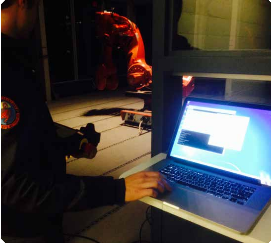
Fig. 3.19. Testing real-time control of chair movements in Labatut with Ryan Johns. A lag between digital simulation movement and robotic movement made live control difficult due to jerky movements and imprecise response. (photo by Charlie Avis).
