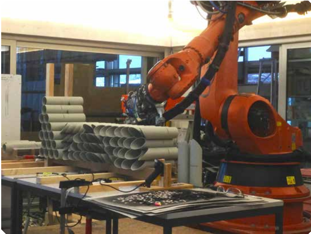
Fig. 1.13. The workspace at the Digital Fabrication lab at the ETH Zurich. The student project is to design acoustic walls controlling three parameters that the robot can manipulate (tube angle, tube length, cut angle). (photo by Charles Avis).
